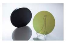
SiC epitaxial wafers are used in nextgeneration power semiconductors, which are expected to contribute to energy saving. These wafers have been increasingly adopted for use in power supplies for data center servers, devices for railroad vehicles, and onboard chargers for EVs.
