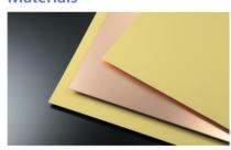
These materials are made by impregnating glass cloth with epoxy resin and then laminating copper foil on both sides. They have high heat resistance, high elasticity and low coefficient of expansion, and are used in printed wiring boards and semiconductor package substrates.
