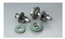
Resonac provides high-strength plastic gears made by processing aramid reinforced fiber sheets into which highly strong and highly heat-resistant polyamide resin has been injected and hardened (product name: "KM-9100"). The gears can be used even under heavy loads and harsh environmental conditions in which conventional plastic gears are unusable.
