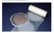
Die bonding films are used to bond IC chips to semiconductor package substrates. The films also contribute to ensuring the reliability of semiconductor packages by mitigating the distortion of the substrates caused by differences in the coefficient of thermal expansion, in addition to providing high bonding strength.
